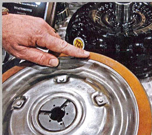
Lock-up converters in OEM automobiles utilize a clutch disc which seats to lock the converter's turbine to the output shaft.
