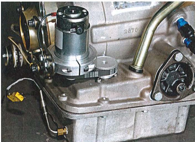
The basis of the SCS-30 is an internal oil pump that is driven by this external motor capable of being used on either 12v or 16v systems. The internal oil pump allows fluid to flow through the transmission even when the engine is turned off.
